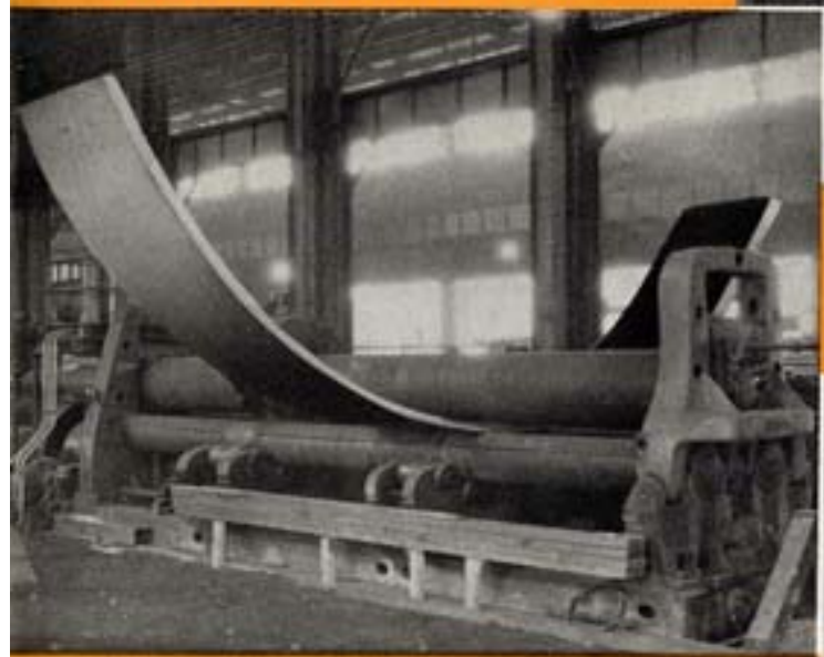
Bending Rolls for plate thickness to 3½ in.
