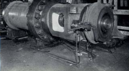
Hydraulic Press being assembled.
