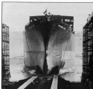
M/V "Shooting Star" Hull No. 101, of C-54 Design, was built for the U. S. Maritime Commission, to be operated by the U. S. Lines. The "Shooting Star" is powered by a 7,200 H.P. Suez Diesel Engine. This vessel was launched December 28th, 1941. The sponsor of the M/V "Shooting Star" was Mrs. Schuyler O. Bland.
