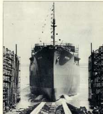
S. S. White Plains — Launched 2:50 P. M. May 30, 1942 — Keel laid December 1, 1941 — Length 303' B. P. — Beam 68' — Depth 37' 3" — Steam Turbine — Built for U. S. Maritime Commission — Sponsor: Mrs. Willard F. Rockwell — (First ship launched in the North Yard).
