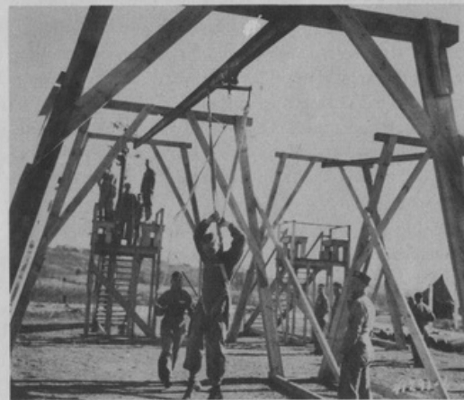
SUSPENDED HARNESS TRAINERS. In this apparatus the parachutist is taught the manual technique of manipulating his parachute during descent, and to tumble upon landing.
