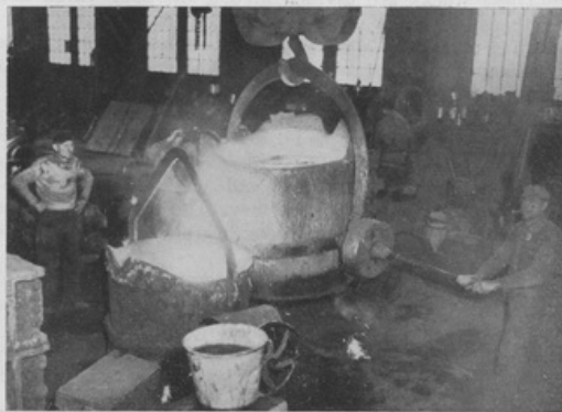
This view shows metal being poured from one large ladle to another. This is done so that the iron can be poured from two ladles into the mold from two sides.
