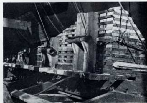
View showing ground ways, sliding ways, and launching poppet, port side, aft.
