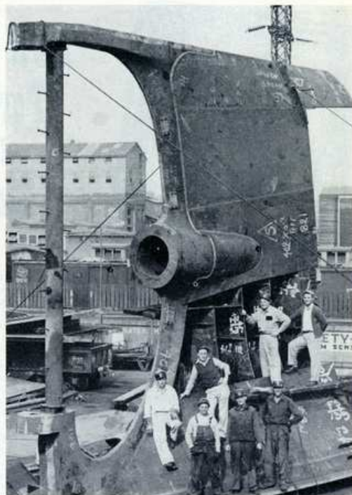
STERN POST ASSEMBLY IN SOUTH YARD — Its massive size dwarfing the seven workers perched on its slopes. Giant cranes swing this into place easily and accurately.
