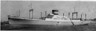
CS — PASSENGER AND CARGO SHIP, PRESIDENT JACKSON — CS F & C — Combination passenger and cargo type, length (over-all) 491' 10", Beam, 69' 6", Draft (loaded), 26' 6", Cruising radius, 20,300 miles,
