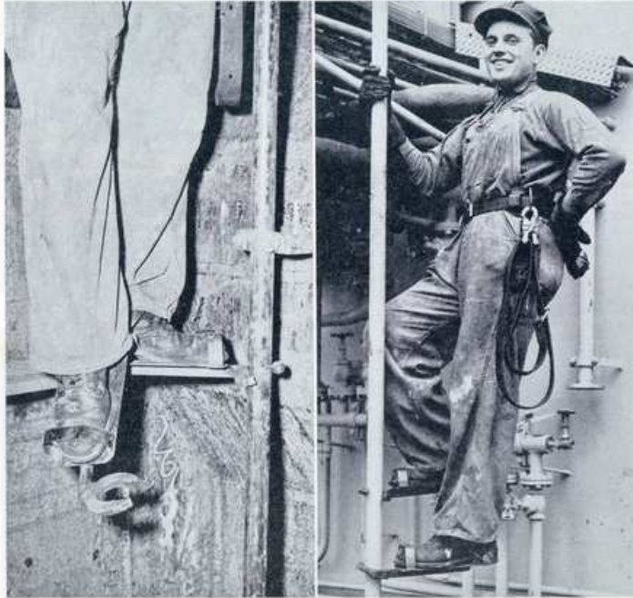
ANTHONY J. PETRUNIS, 34-1035, demonstrates the Pipe Climbing Apparatus for which he was awarded a $100 prize. The photo at left is a detail view. This apparatus is in the form of a pair of shoes which the men put on to climb up the pipes in the tanks after the staging has been taken down. A great deal of time and material is saved, besides increasing the element of safety.
