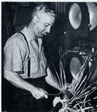
ARMATURE is being assembled by John Wooley, one of the old-timers.
