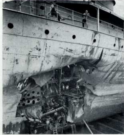
The sturdy "OKLAHOMA" could take it. She survived this blast from an enemy torpedo. Repaired by Sun Ship, she went back to carry war supplies.
