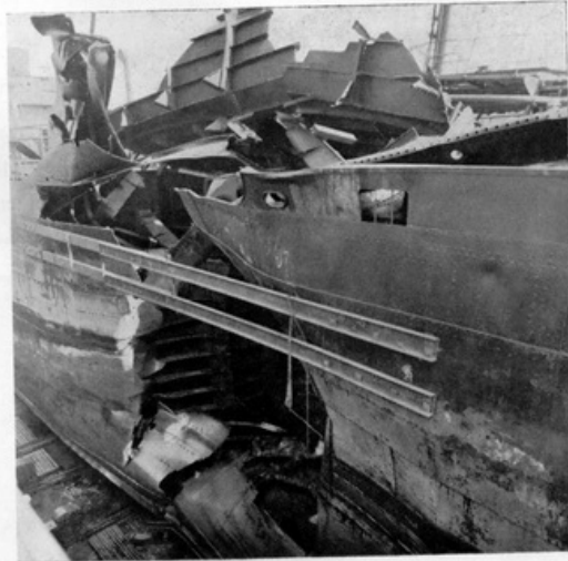
THE VAST CRATER in the tanker which was caused by a torpedo was repaired by experts at Sun Ship's Dry Dock.
