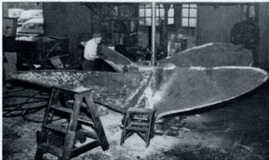
(Left) SECOND STEP — After propeller is bored and faced, it is then ground, chipped and polished as shown in picture by W. Bilsky. All propellers must pass a careful inspection.
