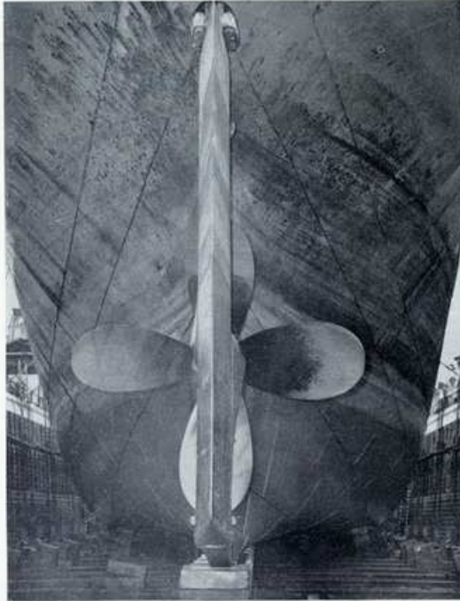
UNUSUAL VIEW OF "CHESTER SUN" showing the huge rudder exactly in line with two blades of propeller.
