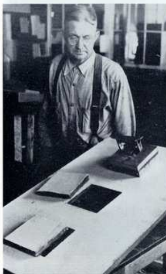
V. H. BURNS is shown with jig which insures the cutting of a neat square hole in insulation.
