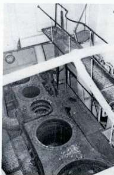
ENGINE PISTONS removed.
