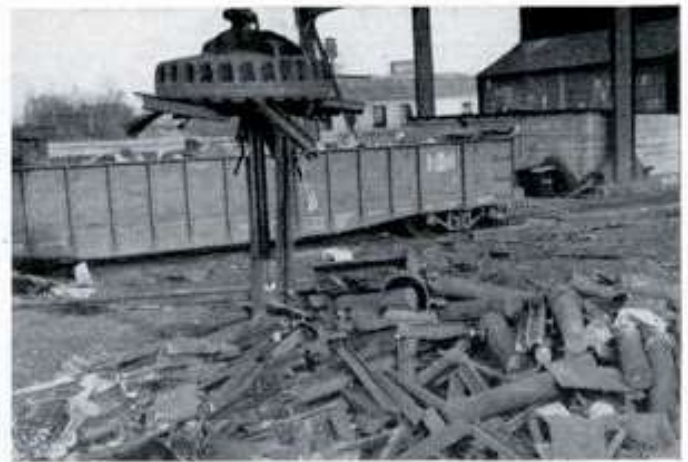
THOUSANDS OF TONS of scrap metal have been collected during the recent "cleaning up" drive. Here is the big magnet in the salvage yard picking up heavy steel rails and other bulky iron and loading it on a freight car.
