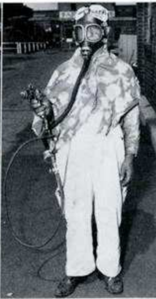
AN AIR-LINE RESPIRATOR with face mask is used when working in confined spaces with a liquid vehicle or solvent injurious to the health.
