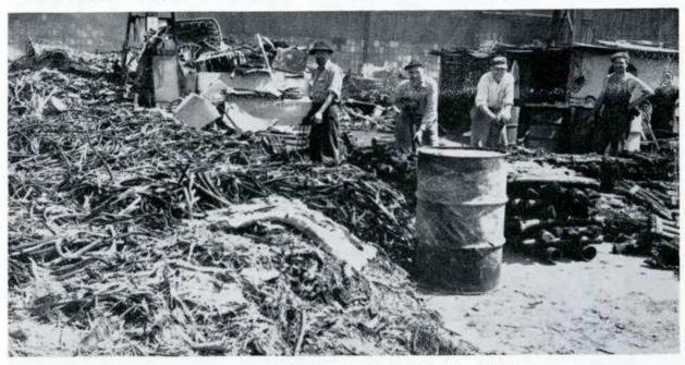
CABLES ARE CUT to short lengths and the insulation is burned off leaving copper salvage. Brass also is reclaimed by these employees. This is one of the steps in the salvaging of ships.
