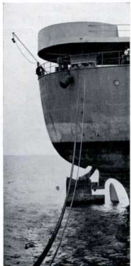
STERN OF SHIP showing how a rudder is hung and also blade of propeller high out of water.
