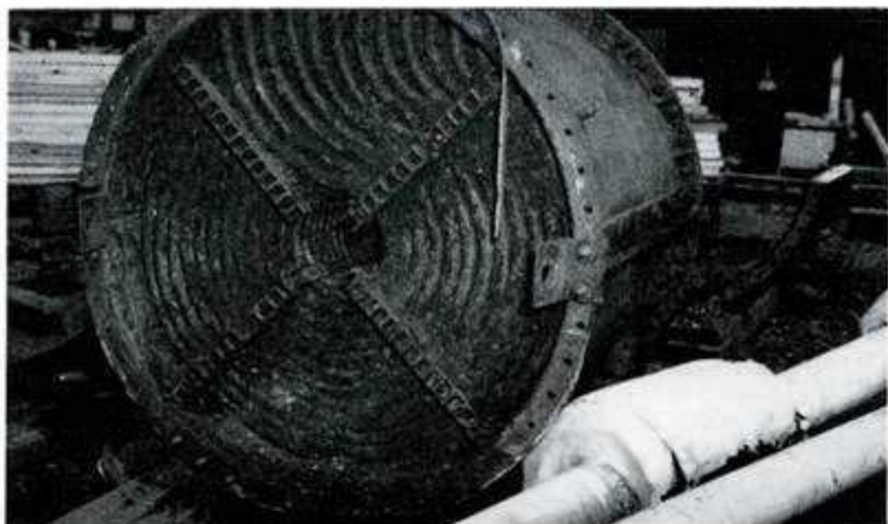
THERE'S HALF A MILE OF ONE INCH COILS in this old section of refrigerating equipment removed from the TIGRE. Sun Ship is installing new refrigeration on the ship and making other improvements.
