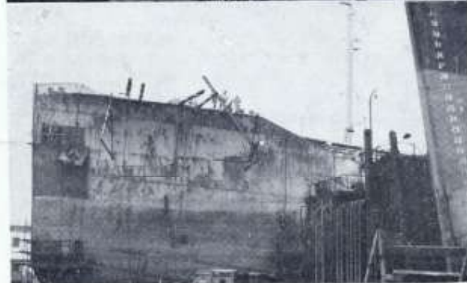
S.S. "JOHN G. WHITTIER" — Liberty ship operated by the States Marine Corporation came to the shipyard for heavy weather damage repairs consisting of drydocking, and realigning the main engine crankshaft, line shaft and tallshaft.
