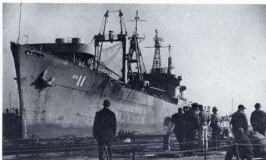
M.S. "STAR BETELGEUSE" ex "Mormaclark" — Built as Sun Hull #180. Purchased from the U.S.M.C. by Compania de la Paloma for operation by Swedish interests. Was towed to the shipyard from the laid-up fleet in the James River for complete examination and overhaul of machinery, removal of Navy installations, drydocking, painting and miscellaneous repairs.
