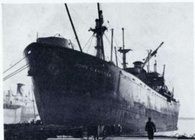
S.S. "WARRIOR POINT" — T2 Tanker purchased from the U.S.M.C. by the Overseas Tankship Corporation. Removal of defense features, alterations to quarters, drydocking and installation of shell and deck straps.
