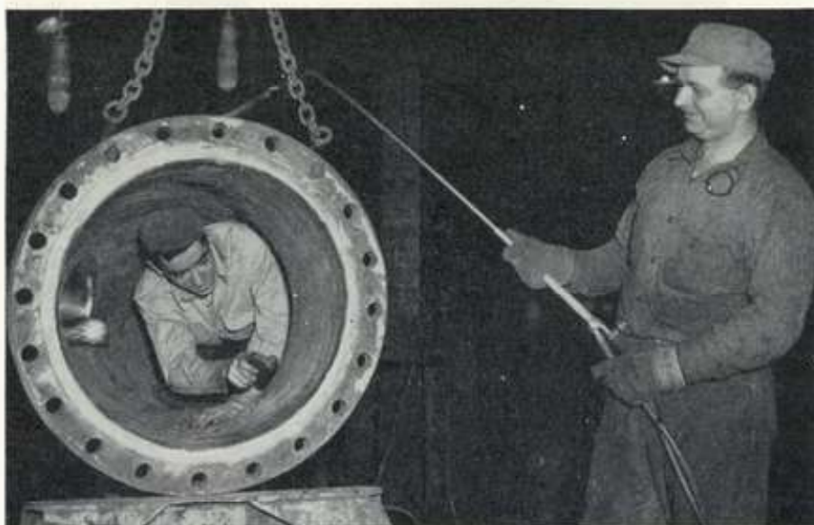
OUT OF ORDINARY TASK at Copper Shop is putting a coating of solder on the inside of large pipes. Here you see W. Davis, inside a pipe wiping solder, while A. Adam, Jr. heats the outside sufficiently to melt the solder.
