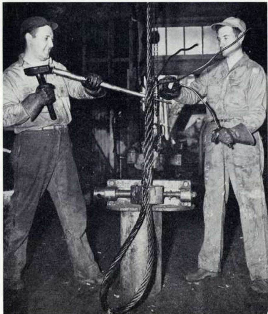
SPLICING AN EYE in wire is a heavy job. William Murtaugh and Howard Ebright show how it is done.
