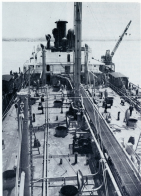
BACK OF TANKER is a photograph arrangement of pipes, valves, vents, tank openings, vehicles and other gadgets, running down the center of the tank in the "catwalk."
