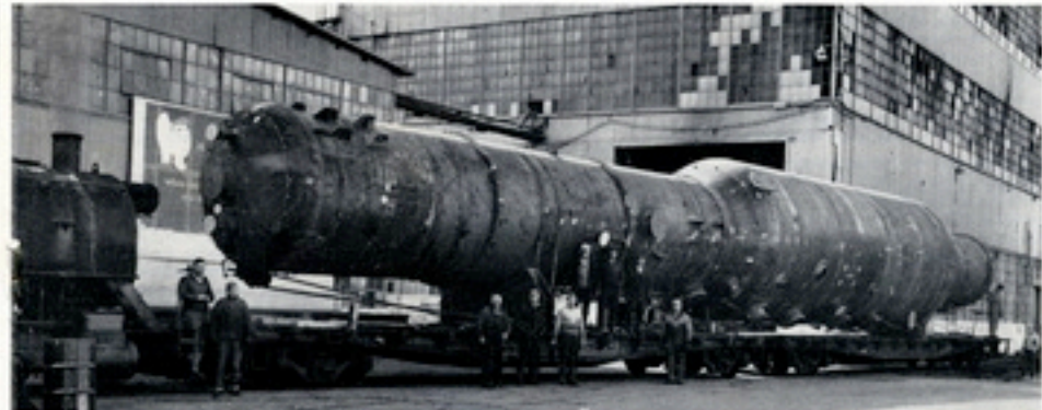
UNUSUAL AND VERY COMPLICATED PIECE OF STEEL WORK. It is a fractionating tower with shell in three different diameters, the largest diameter being 12' 6". Inside the overall length is more than 100 ft. There are many nozzles, brackets and connections, a cone transformation section reducing the shell from the large to a smaller section. Also the inside of this vessel is full of special trays which are very intricate and difficult to make. The vessel's size is beyond normal rail clearance limits. It was moved over the Pennsylvania Railroad by a special train movement in all daylight and at slow speed from Sun Ship to Bayonne, New Jersey. The tower is shown just as it was moved from the Boiler Shop where it was built in record time.
