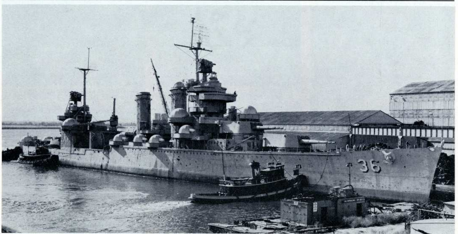
LAST STOP ON LONG AND ILLUSTRIOUS TRIP from shipway to scrapyard is made by heavy cruiser Minneapolis. Tugs nose her in to scrapping pier in Our Yard where she will be cut into small pieces to be sold as scrap. Of the CA 36 class, she is 588 feet long, 61' 9" across and has a mean draft of 19' 5". Displacement is 9,950 tons. Armament is nine 8-inch guns, eight 5-inch anti-aircraft batteries and a host of lesser arms. Her full complement was 700 men. She has eight boilers in four engine rooms which developed 107,000 horsepower and she could breeze along at 32.7 knots. But, as her nameplate shows, she was built in 1933 which is horse-and-buggy days for war materiel, so it's "Goodbye, Minneapolis!"
