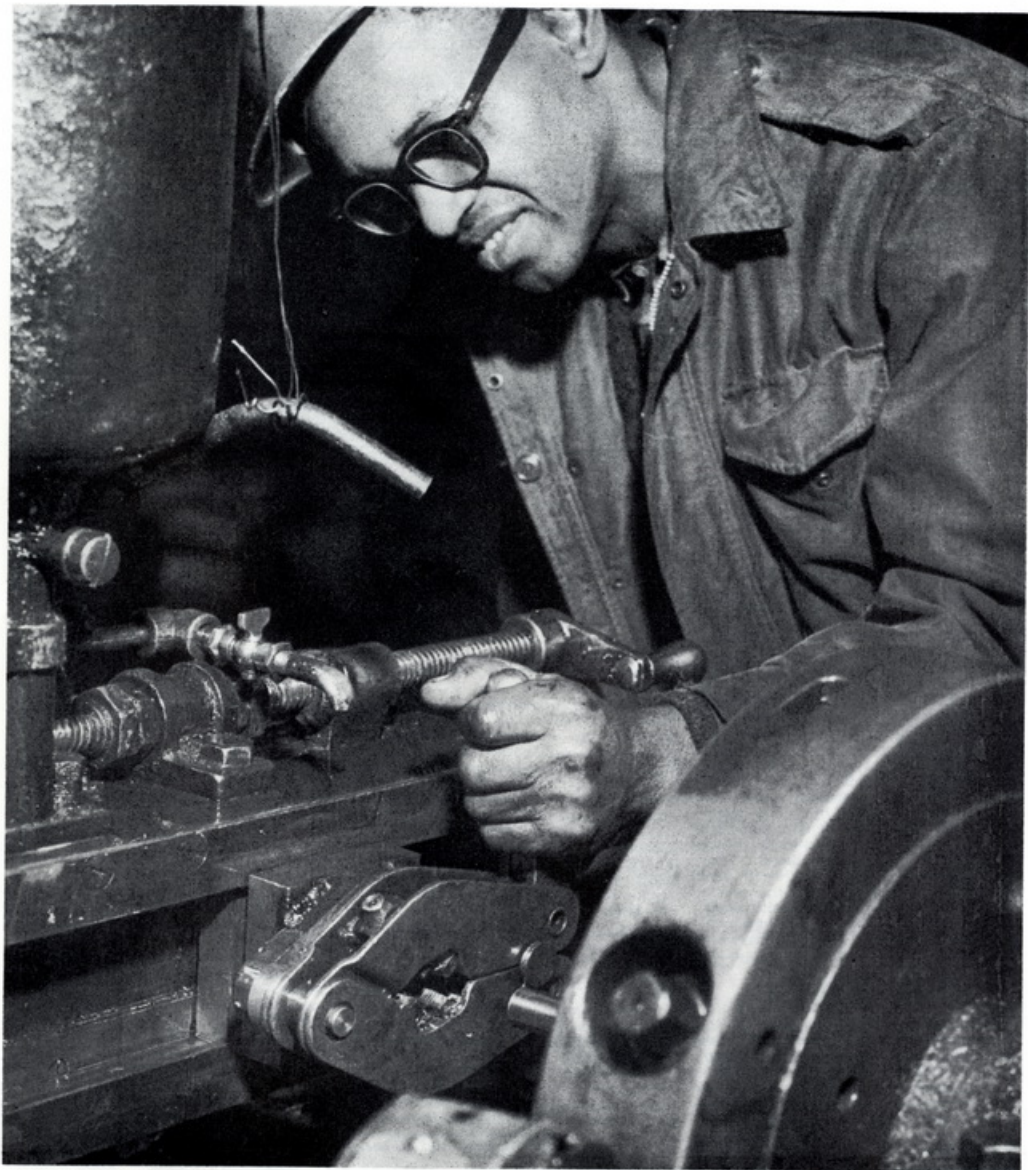
LITTLE DIAMOND SHAPED CLAMP under hand of William Briggs (34-289) meant difference between "use" and "scrap" to a lot of chromium pipe. This thread cutting machine held pipe tightly but die couldn't do job on tough chromium. Other dies that would didn't fit machine. Bill had this jig made. You can see upper and lower parts of die through opening. Bill pulls down handle in his hand when pipe is in place clamping jaws of jig and pressing die firmly in contact with pipe. When job is done he flips up handle and pipe can be slipped out. Read about it on page 4.
