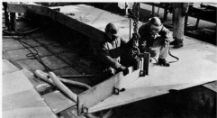
Crafts work closely to meet schedules. On the left is Marion Davis, a fitter, with Alex McDonald, a welder, as together they prepare a web frame for welding.
