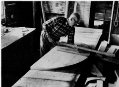
Patternmaker Frank Weaver is one of the men who make the templates to later be used in any number of shipbuilding operations.
