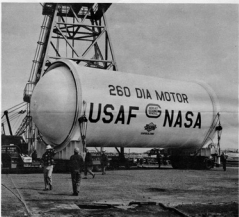
A Sun Ship product, this solid fueled rocket motor case is the largest ever successfully built and fired.
