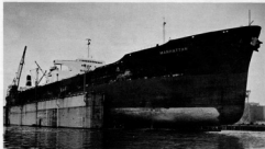
MANHATTAN, the largest U. S. merchant vessel, is now at Sun Ship for conversion of the bow to an icebreaker. The 114,000 dwt MANHATTAN can transport over 38 million gallons of oil, a capacity that would require a railroad tank car train 27 miles long to carry. Note how it extends over the dry dock.
