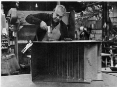
A Sun Ship craftsman in the Sheet Metal Shop prepares the ventilation turning vanes for a piece of ducting.
