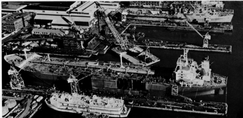
Aerial View Shows Magnitude of Ship Repair Work on Manhattan Duke. Repairing the 220 ft. long hole in the tanker's port side required 1230 tons of steel, a shipyard record for a damaged vessel in terms of steel weight replacement.
