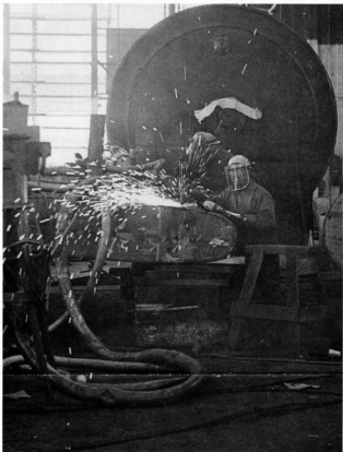
Sparks fly as William Helton grinds the rough spots from the rudder of Hall 677.
