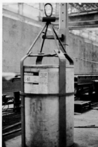
Show here is the Conrac unit's new wire barrel lifter that was installed. The 1,000-pound barrels are now being lifted under safer conditions.
