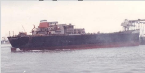
6.5: The ship's house had to be built in two sections due to lack of clearance on the shipway No.2's 'Bridge' cranes. The section with the ship's stack (left side) is the upper deck section that will later be lifted into place at the Philadelphia Navy Yard. Photo courtesy of Dave Boone SSHS:326_50_009_db
