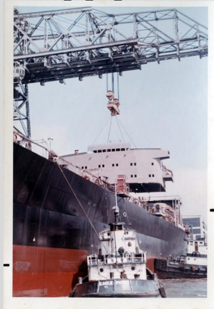
6.7: The 'American Astronaut' container ship underway. Note the two vertical 'columns' aft of the 'house', these are the actual ship's 'smokestacks'. Photo courtesy of Dave Boone SSHS: 453_47_035a [10]
