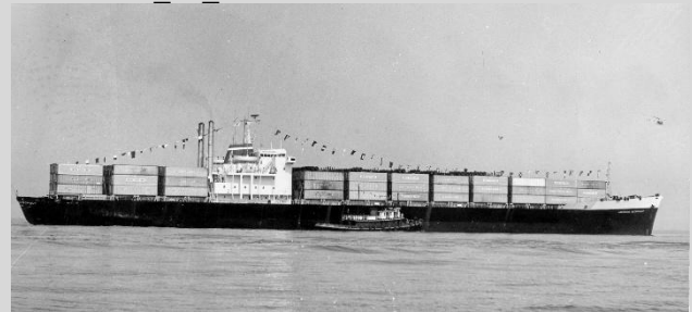
6.7: The 'American Astronaut' container ship underway. Note the two vertical 'columns' aft of the 'house', these are the actual ship's 'smokestacks'. Photo courtesy of Dave Boone SSHS: 453_47_035a [10]
