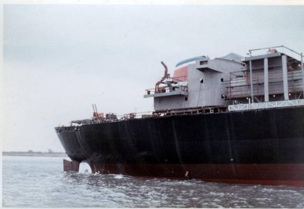
6.5: The ship's house had to be built in two sections due to lack of clearance on the shipway No.2's 'Bridge' cranes. The section with the ship's stack (left side) is the upper deck section that will later be lifted into place at the Philadelphia Navy Yard. Photo courtesy of Dave Boone SSHS:326_50_009_db
