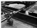
A "travagance" in 47 shop was used to burn out the bismarck diffuser. As the electric fireproofing follows the template, the bright burning beads (background) zip-zap down the plate, cutting the nested pieces.
