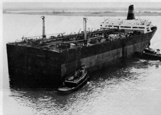
Stern section as it was towed to wet basin.
