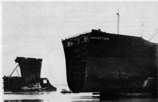
Bow (left), separated from the forward hull structure, is towed away.
